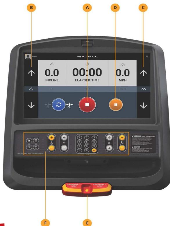
A) GO/STOP: One touch start (displayed on-screen before workout). Press to end workout and show workout summary data.
